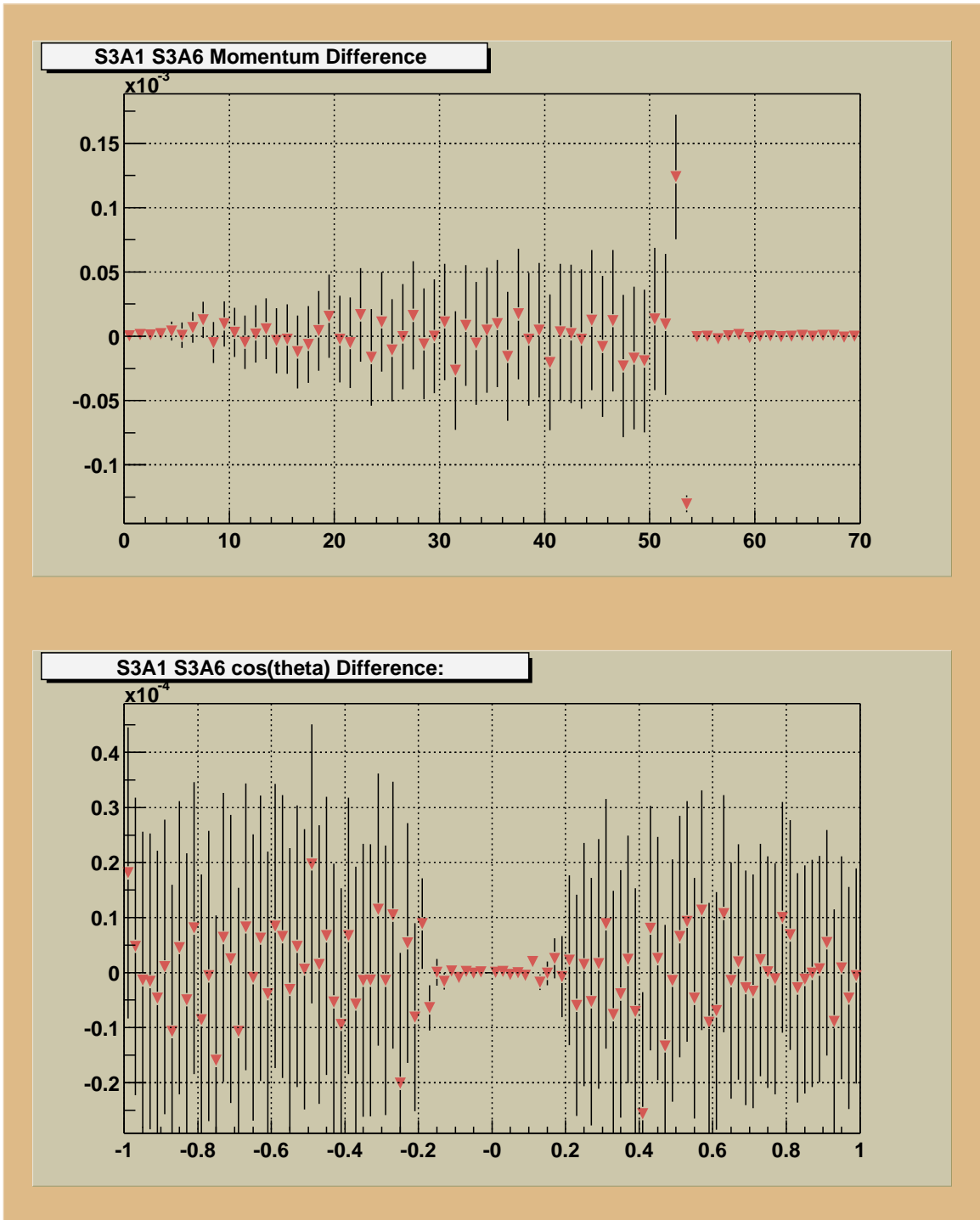
Figure 2: Momentum difference (top) and \cos(\theta) difference (bottom) for the analysis of set3 using nominal plane positions in one analysis and randomly shifted UV plane positions in the second.
